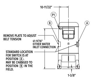
**Note:** Approximate shipping weight of peeler and peel trap unit: 201 lbs. Net weight of peeler and peel trap unit: 190 lbs.
