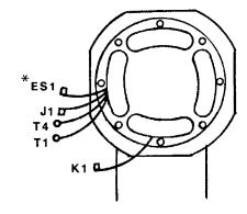
\* ES1 IS ONLY ON STATORS **ABOVE 150 VOLT WITH ELECTRONIC START SWITCH**
