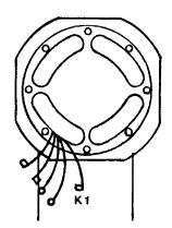
If mixer has a mechanical start switch, position stator as shown.
