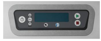
The digital controls are placed in a convenient panel that lets operators verify proper operation and temperatures at a glance. The digital display indicates the unit is on, and confirms that the doors are closed. Automatic door interlocks prevent the pump and conveyor from operating if the doors are open. Easy to read display indicates accurate temperatures of the 150°F wash, 160°F power rinse, 160°F dual rinse and 180°F final rinse.
