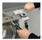
**1. UNLATCH & OPEN COVER.** Wait until shaft has stopped turning.
