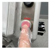
**3. PRESS RED STOP BUTTON.**A built-in brake will quickly stop the attachment shaft when power has been turned off.
