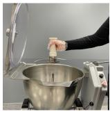
5. INSERT ATTACHMENT. Slide attachment onto center shaft. Rotate until it drops down over square part of center shaft. Be sure attachment drops completely into place.
