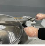
2. UNLATCH COVER. Holding cover handle in left hand, pull the cover latch toward you.
