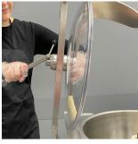
8. ATTACH BAFFLE HANDLE. Hold baffle handle with lock knob upright and large knob of baffle handle at bottom, and slide round pin over the mixing baffle shaft and into groove.
