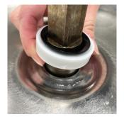
**10. REMOVE & CLEAN BOWL SEAL ASSEMBLY.** Bowl seal and retainer ring snap on and off without tools for cleaning.
