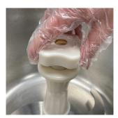
6. LOCK ATTACHMENT. Use the twist lock knob furnished. Place knob over shaft and twist until tight.
