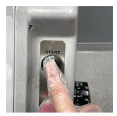
PRESS START SWITCH & HOLD. Machine will run until switch is released.
