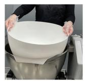
**1. INSERT STRAINER BASKET.**Do not use with mixing baffle.
