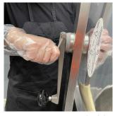
9. LOCK BAFFLE. Rotate lock knob downward until it stops.
