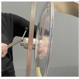
3. REMOVE MIXING BAFFLE.
