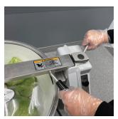
11. LOCK COVER. Grasp cover handle and pull cover down into closed position. Press cover handle down before rotation cover latch away from you.
