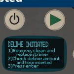
**INSPECT THE INTERIOR OF THE** MACHINE. If necessary, another delime cycle can be initiated by entering the **Manager Programming Mode** (repeat steps 1-4 above).
