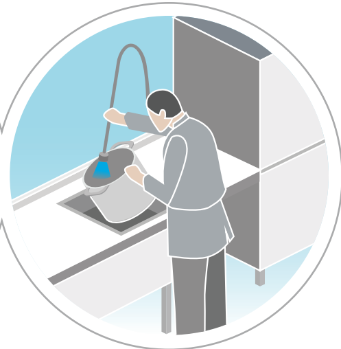
Condensing steam in the dishwasher reduces latent and sensible in dishroom and eliminates the need for a costly vent hood.
